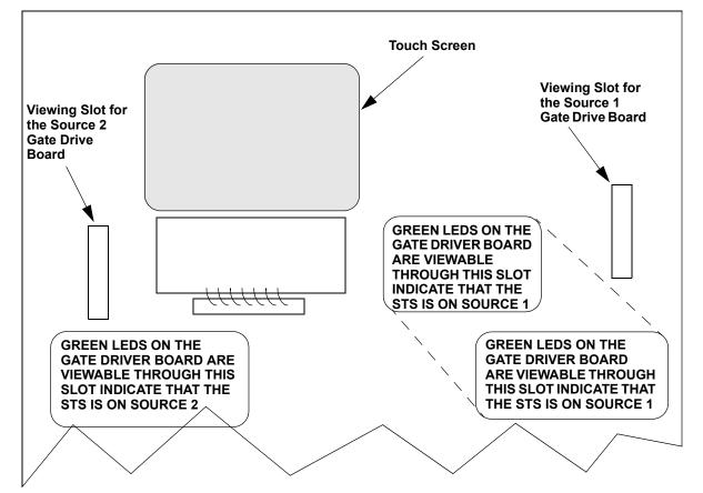
If the Color Graphical Display is not available, you can still use the following bypass procedures, ignore the steps to check the display and check the LEDs.
